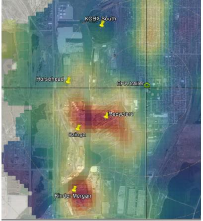
Figure 6. Manganese polar plot, concentration (ng/m<sup>3</sup>) averaged by wind direction and speed
