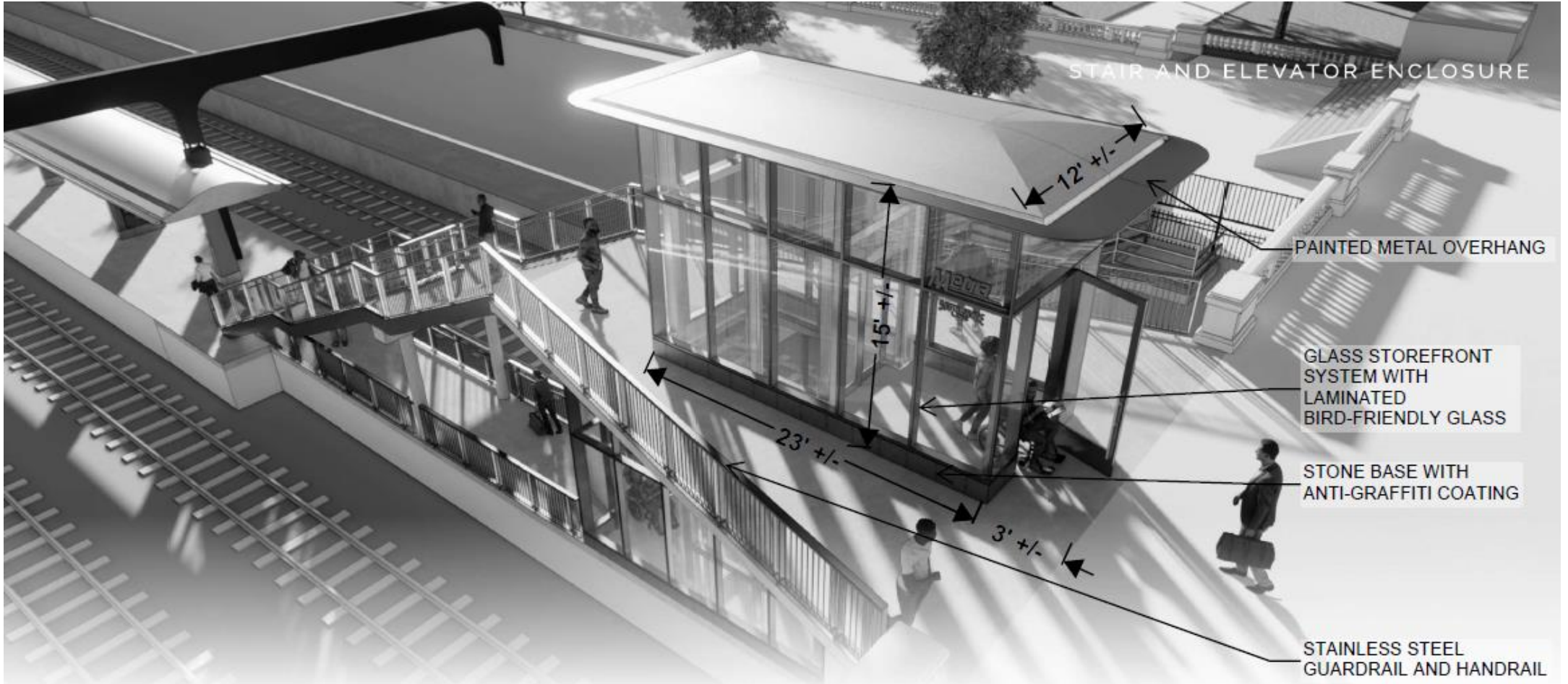
JACKSON DRIVE NEW ELEVATOR AND STAIRWAY
